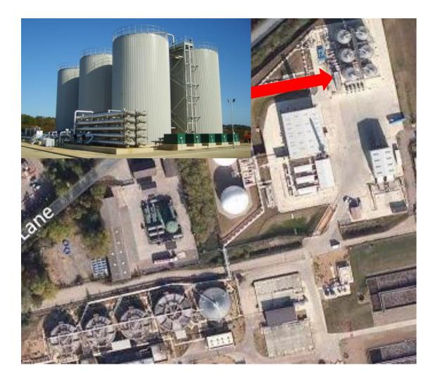
40,000 TDS p.a. WWTW (~12,000 TDS indigenous, ~28,000 TDS imported) Solution as part of an integrated power and sludge upgrade 4 existing digesters retained 4.2MWe CHP capacity
