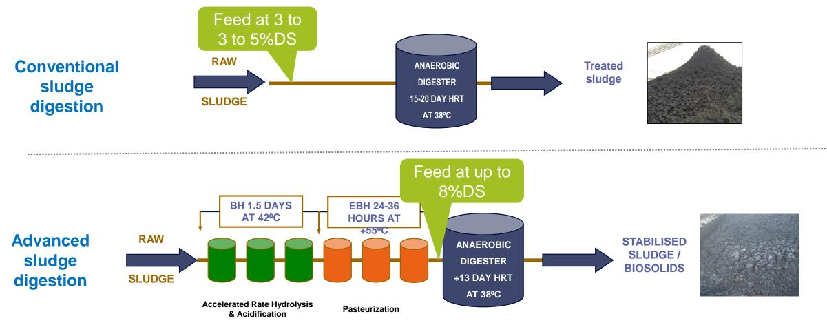
Critical factor - All advanced digestion pre-treatment systems allow for significant increase in digester dry solids feed
